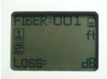
4. Press the “Meas” key, the fault location or link distance, and link loss are shown. The unit in m or ft can be selected by pressing the “Unit” key.
