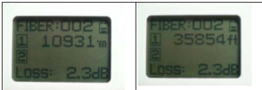
5. Save the current data of line number, fault location, link distance, and link loss by pressing the “Save” key. The stored data for each fiber number can be recalled by pressing the ▲▼ key till the required fiber number appears.
