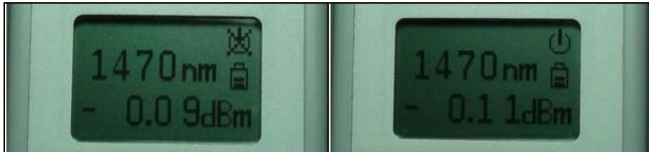
4. The power unit is normally in dBm. When the dB/dBm key is pressed for about 3 seconds until dB is flashing on the LCD, the current input power level is taken as the new reference at 0 dB, and the following measurement will be the difference in dB, with respect to the new reference. The reference value is stored in the unit even after the unit is turned off. A new reference can be set by pressing dB/dBm key again. The unit can also be selected as mW,  $\mu$ W, or nW by pressing dB/dBm key.
