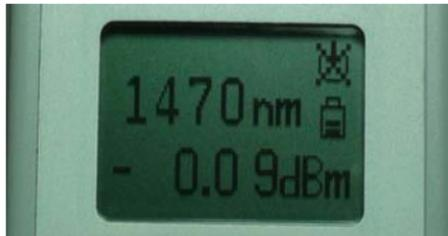
2. Press  $\lambda$  -key until the correct input wavelength is displayed. The displayed power value is the measured value. Press the  $\blacktriangledown$  ( $\lambda$  s) key to display all the eight wavelengths with power values.
