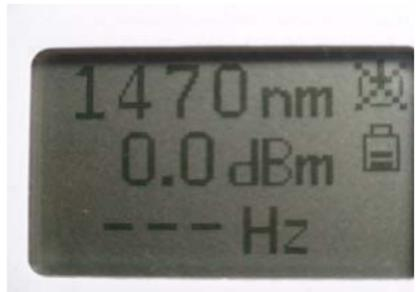
2. The auto-off feature can be disabled by pressing the “Auto Off” switch, as indicated by the power symbol without a cross.
