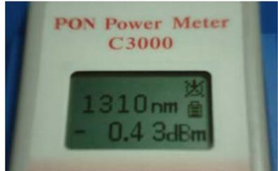
2. Press  $\lambda$  -key until the correct input wavelength is displayed. The displayed power value is the measured value. Press the  $\blacktriangledown$  ( $\lambda$  s) key to display all the three wavelengths with power values.
