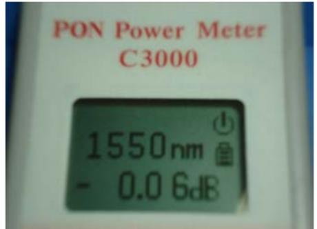
4. The power unit is normally in dBm. When the dB/dBm key is pressed for about 3 seconds until dB is flashing on the LCD, the current input power level is taken as the new reference at 0 dB, and the following measurement will be the difference in dB, with respect to the new reference. The reference value is stored in the unit even after the unit is turned off. A new reference can be set by pressing dB/dBm key again. The unit can also be selected as mW, uW, or nW by pressing dB/dBm key.
