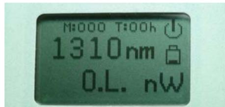
4. The measured value can be stored in the memory address M:xxx sequentially by pressing S/C key. YES or NO is selected by the  $\blacktriangle$  and  $\blacktriangledown$  keys. If YES is selected, by pressing the S/C key again, the data is stored in the memory address as shown. If NO is selected, by pressing the S/C key again, the screen is back to measuring mode without storing the data.
