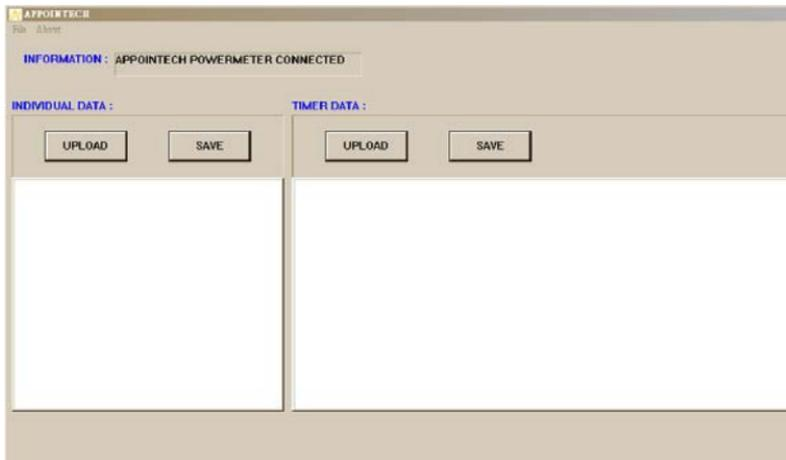
**STEP 4 :** Press **MENU** button on C2000 and select “**UPLOAD**” on the LCD with **▼** key, press **MENU** button again; The LCD shows USB ready. If USB NOT READY is shown, repeat from STEP 1.
