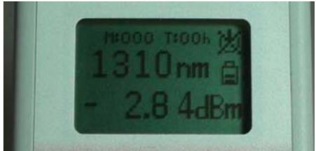
Press  $\lambda$  -key until the correct input wavelength is displayed.
