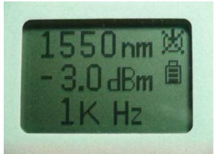
3. Press Hz switch for modulated output at 270, 1K, or 2KHz.
