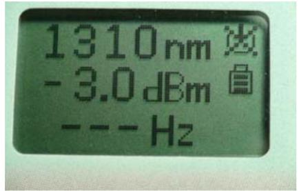
2. Press  $\lambda$  switch to select 1310nm or 1550nm output wavelength.
