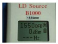
The auto-off feature can be disabled by pressing the "Auto Off" switch, as indicated by the power symbol without a cross.
