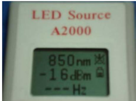
2. Press  $\lambda$  switch to select 850nm or 1300nm output wavelength.
