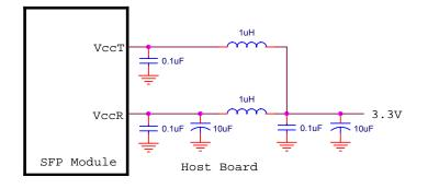
Example SFP Host Board Schematic
