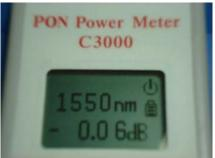
4. The power unit is normally in dBm. When the dB/dBm key is pressed for about 3 seconds until dB is flashing on the LCD, the current input power level is taken as the new reference at 0 dB, and the following measurement will be the difference in dB, with respect to the new reference. The reference value is stored in the unit even after the unit is turned off. A new reference can be set by pressing dB/dBm key again. The unit can also be selected as mW, uW, or nW by pressing dB/dBm key.
