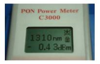
2. Press  $\lambda$  -key until the correct input wavelength is displayed. The displayed power value is the measured value. Press the  $\nabla(\lambda s)$  key to display all the three wavelengths with power values.
