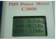
The "low" indicates power <-60dBm. The power readings at two adjacent channels are the small cross-talk from 1550nm.
