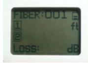
Press the "Meas" key, the fault location or link distance, and link loss are shown. The unit in m or ft can be selected by pressing the "Unit" key.
