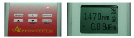
2. Press  $\lambda$  -key until the correct input wavelength is displayed. The displayed power value is the measured value. Press the  $\mathbf{\nabla}(\lambda \mathbf{s})$  key to display all the eight wavelengths with power values.
