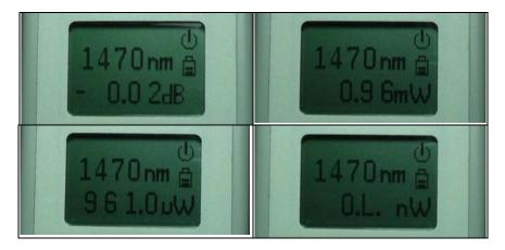
5. When battery power is too low to assume proper operation, an empty battery symbol is shown on the LCD display. When charging is required, plug in the USB connector of the power adaptor (100~240VAC). When charging in OFF-mode, the indicator LED is on until charging has been completed. It takes about 4 hours to get full charge.
