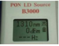
2. Press  $\lambda$  switch to select 1310nm, 1490nm or 1550nm output wavelength.
