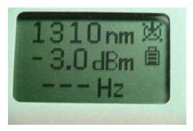
2. Press  $\lambda$  switch to select 1310nm or 1550nm output wavelength.
