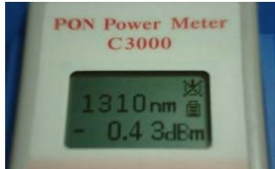
2. Press  $\lambda$  -key until the correct input wavelength is displayed. The displayed power value is the measured value. Press the  $\nabla$  ( $\lambda$  s) key to display all the three wavelengths with power values.
