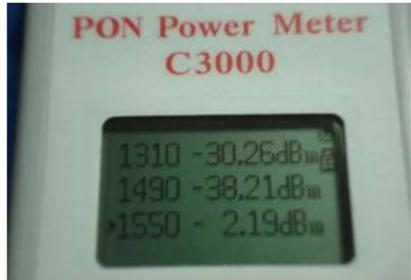
The "low" indicates power <-60dBm. The power readings at two adjacent channels are the small cross-talk from 1550nm.
