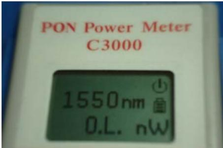
5. When battery power is too low to assume proper operation, an empty battery symbol is shown on the LCD display. When charging is required, plug in the USB connector of the power adaptor (100~240VAC). When charging in OFF-mode, the indicator LED is on until charging has been completed. It takes about 4 hours to get full charge.
