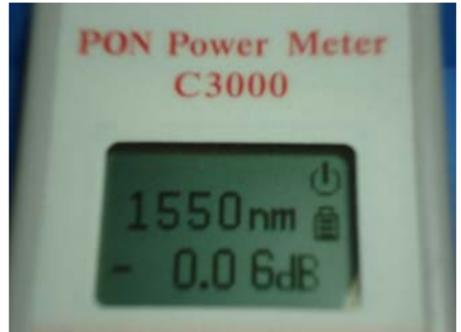
4. The power unit is normally in dBm. When the dB/dBm key is pressed for about 3 seconds until dB is flashing on the LCD, the current input power level is taken as the new reference at 0 dB, and the following measurement will be the difference in dB, with respect to the new reference. The reference value is stored in the unit even after the unit is turned off. A new reference can be set by pressing dB/dBm key again. The unit can also be selected as mW,  $\mu$ W, or nW by pressing dB/dBm key.
